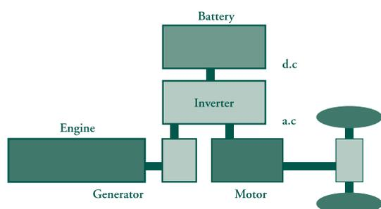
*Figure 3: Parallel Series Hybrid System*
