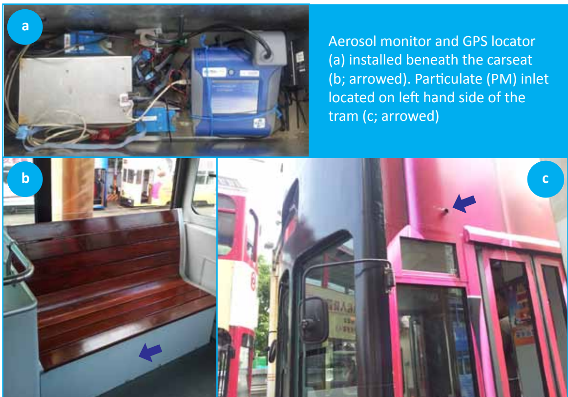
Figure 1. Air quality monitoring unit on the tramcar
