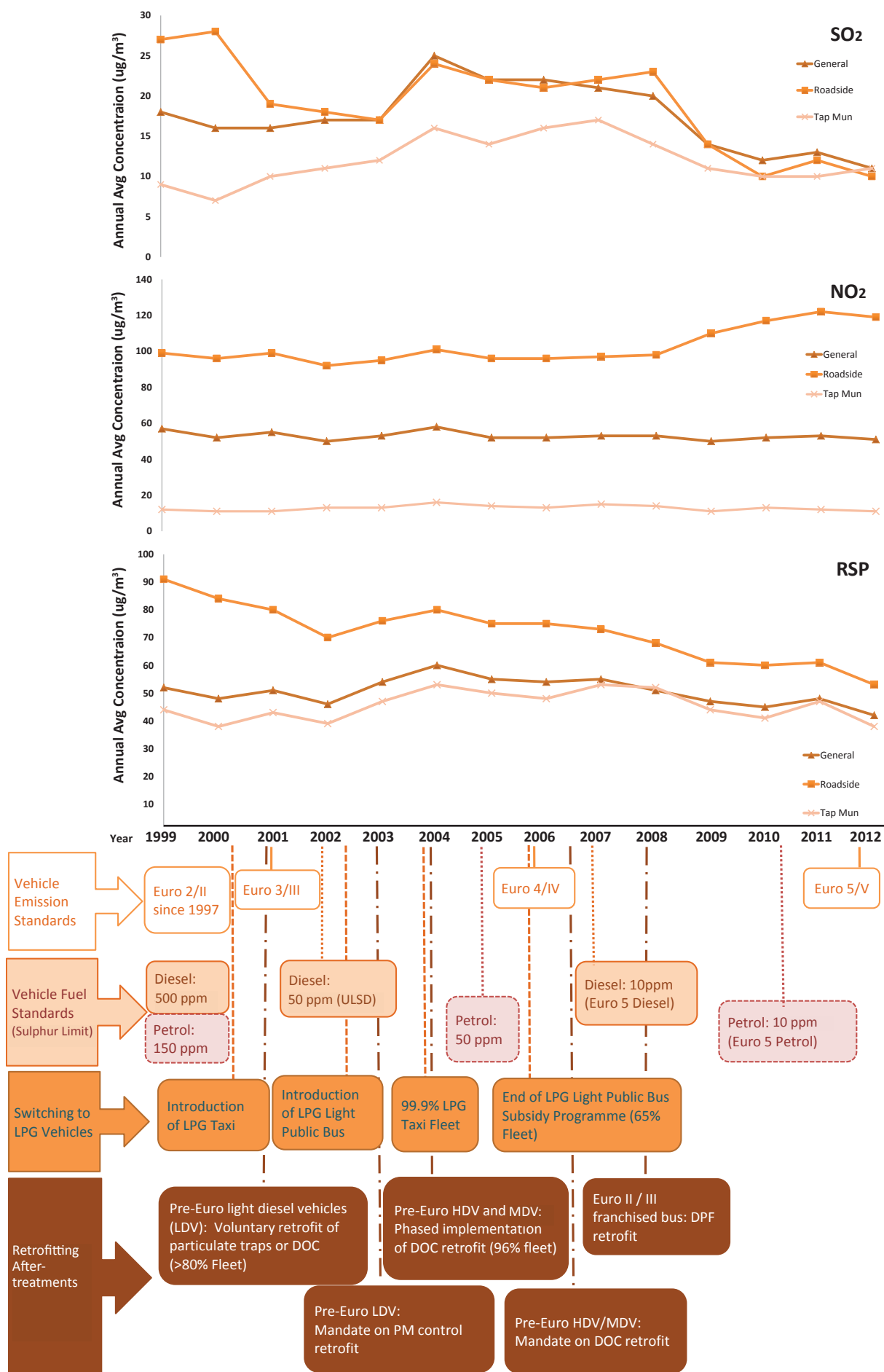
Figure 1A: Air pollutant concentration and vehicle emission control measures implemented to date (SO 2 , NO 2 and RSP)
