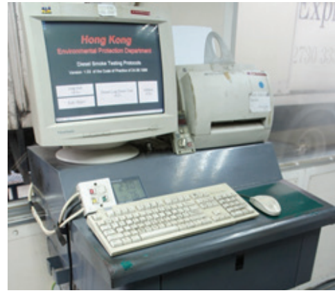
Figure 2: The dynamometre and the computer used for conducting the Lug-down test at VETC in Yuen Long
