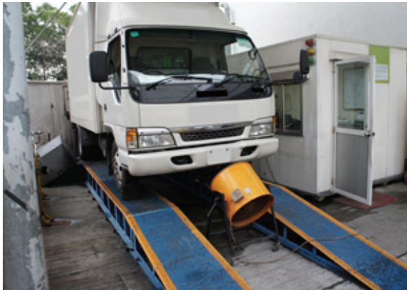
Figure 2: The dynamometre and the computer used for conducting the Lug-down test at VETC in Yuen Long
